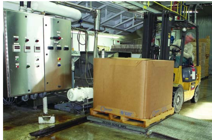
A worker places an IBC tote upon a scale, where it remains while the maple syrup is poured inside the inner bag until reaching target weight.
