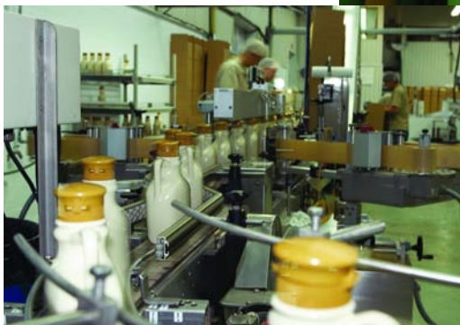
Plastic 32-ounce jugs of maple syrup speed down the plant's bottling line on their way to the labeling station.
