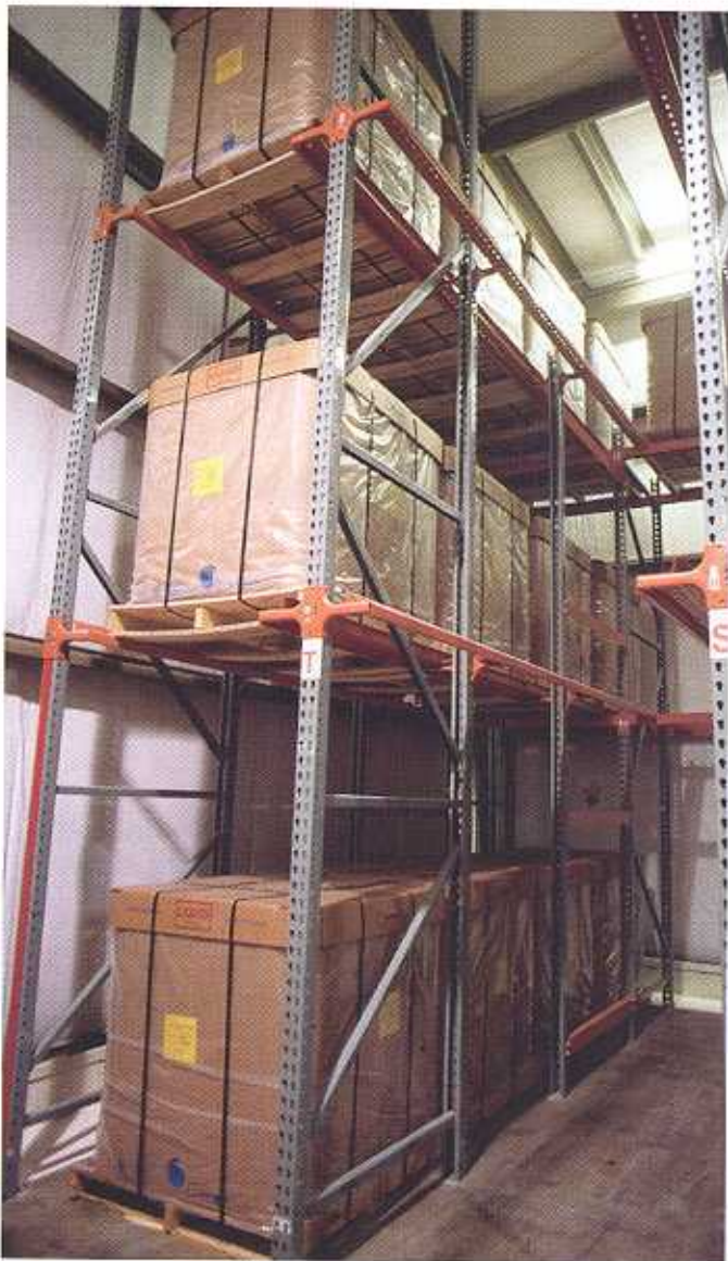
The sturdy IBCs can withstand up to 30 tons of compression and can be racked or stacked as-is up to four-high.
