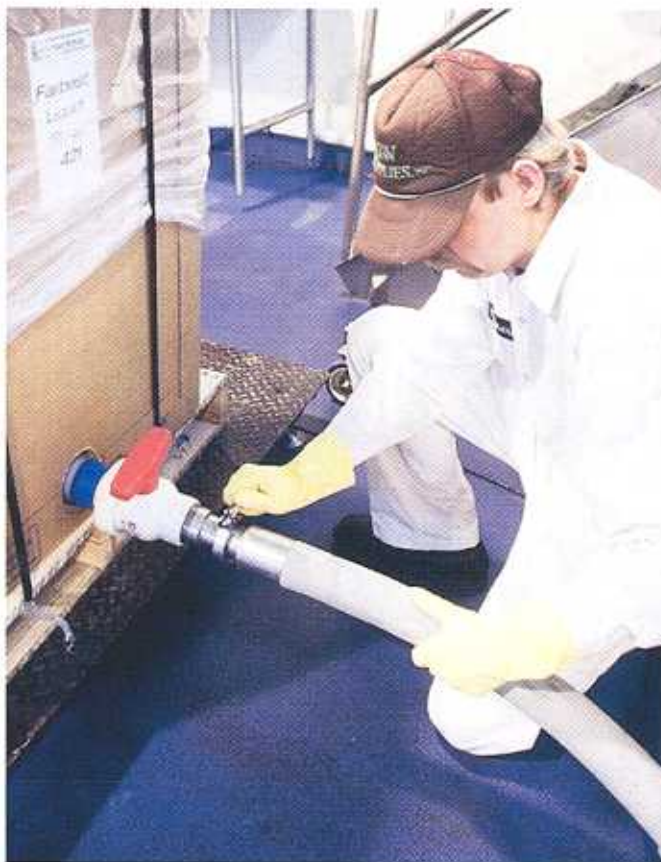
Farbest also receives raw materials in the IBC. An operator attaches a fill hose to the bottom dispensing valve of an incoming container and opens the valve to release product that pumps to a recirculating tank.
