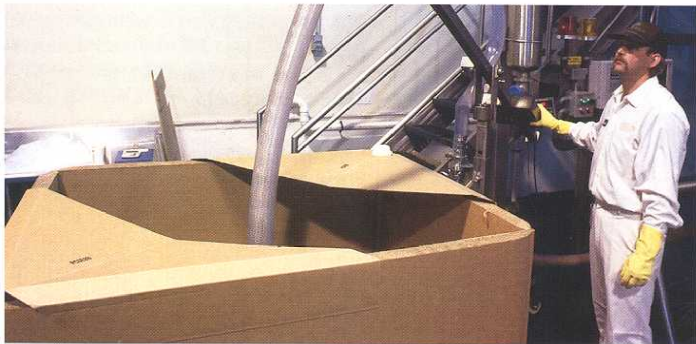
Directly above, the 260-gallon IBC is being filled by way of an articulating arm that permits automatic filling and cuts labor. The 2-
