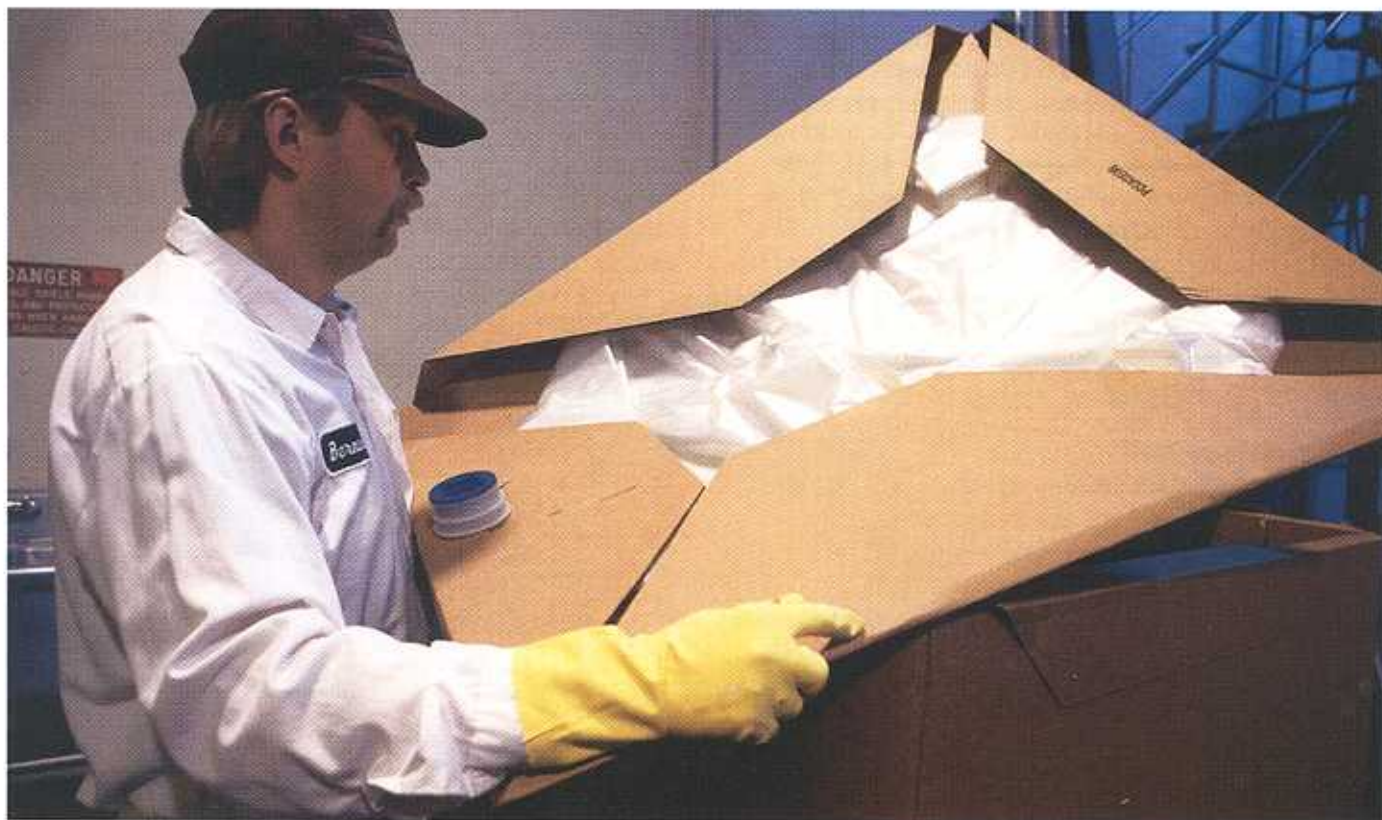
The bag liner is supplied in a corrugated cassette that can be easily inserted into the outer corrugated sleeve.
