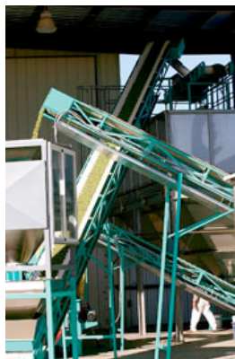
Olives ride a bulk elevator from the groves to processing area of the plant.
