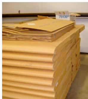
The IBCs are supplied to COR flat, above, stacked 12 to a pallet. The corrugated cassettes with new liners are also sent. The flat stacks take up minimal storage space.
